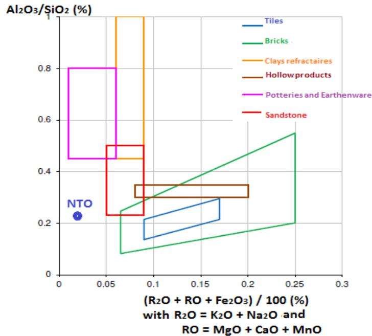
Fig. 12: Positioning of NTO sample in Augustinik diagram
