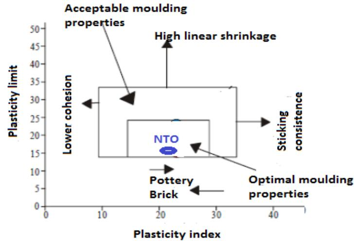
Fig. 7: NTO sample in clay workability chart (Bain and Highly, 1978)
