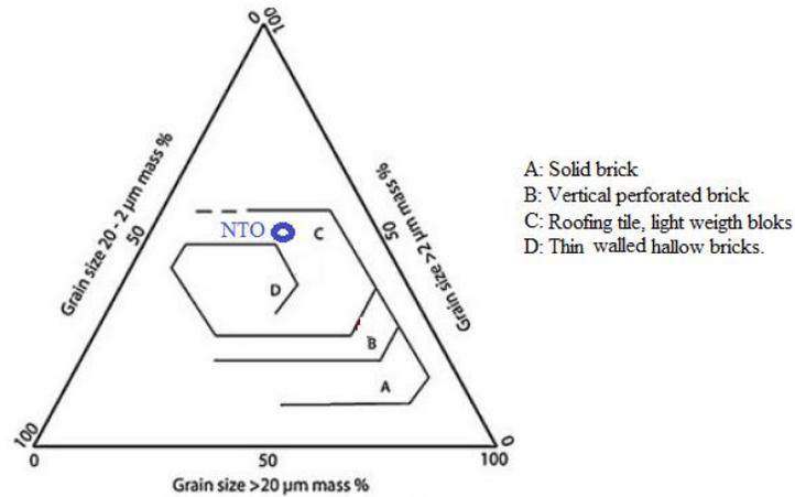
Fig. 4: Positioning of NTO sample in Winkler diagram (Capitâneo *et al.*, 2005; Dondi *et al.*, 1998; Monteiro and Vieira, 2004)
