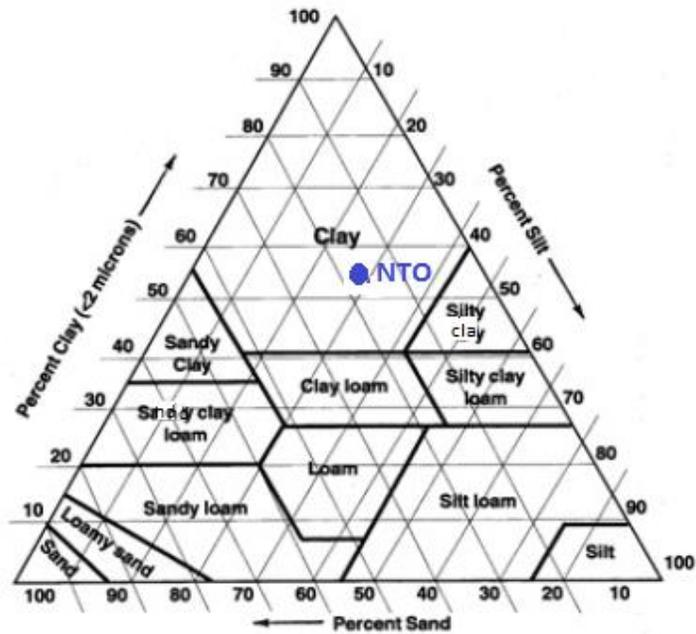
Fig. 3: Positioning of NTO sample in Taylor diagram (United States Department of Agriculture, 1993)
