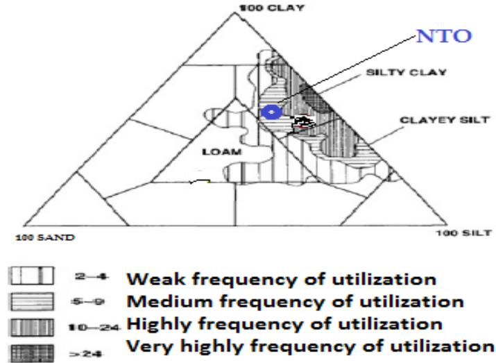
Fig. 5: Positioning of NTO sample in Shepard diagram (Dondi *et al.*, 1998)
