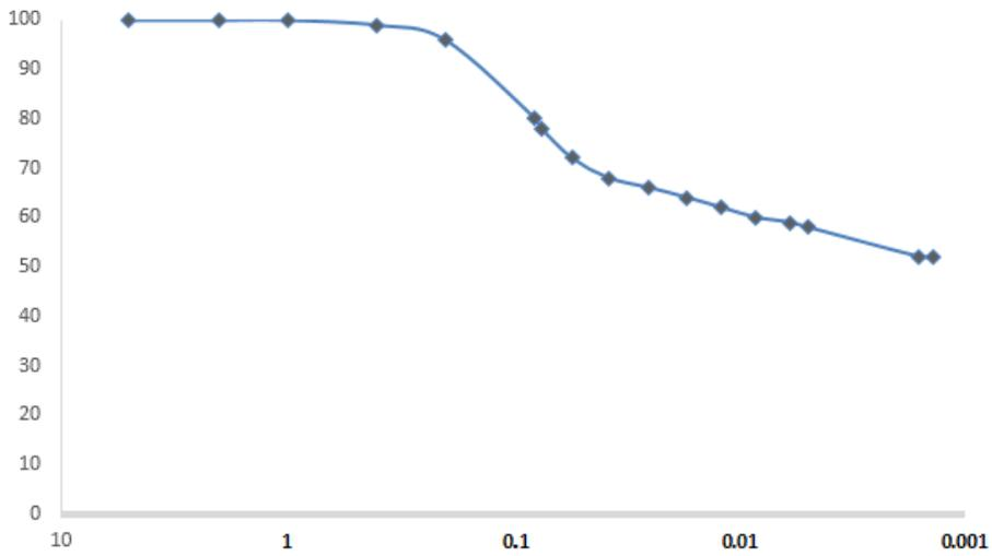
Fig. 2: Granulometric distribution of Ntokou clay
