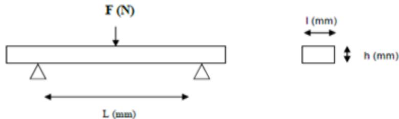
Fig. 1: Flexural strength
